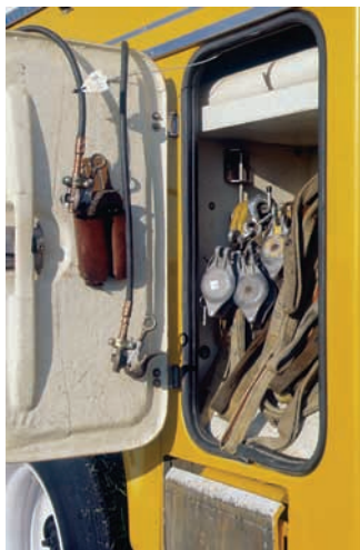
A lineman uses a personal grounding set when working on energized lines. The metal pulleys, running blocks and web slings are used when stringing electric lines.
