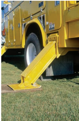
Outriggers stabilize the truck during work on lines.
