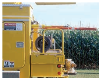
The longer pole is an extendo stick, which is used for moving live electrical equipment. The hot stick next to it helps connect devices such as transformers to energized lines.
