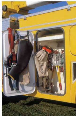
While working in a bucket truck, a lineman wears a safety harness that snaps to a hook in the bucket. If he falls out of the bucket, the harness would stop his fall. Other safety items such as rubber liner gloves and arm protector sleeves are stored in this area too.
