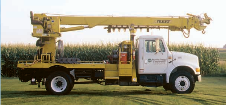
This 1998 Model 4900 International digger derrick cost $135,000 when it was new. It's used primarily to dig holes and set poles. Some electric co-ops add a bucket and use rigs like this one for security light repair and maintenance tasks on pole-mounted electrical equipment.
